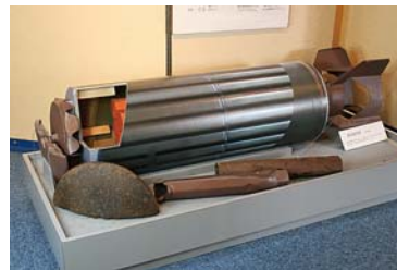
Actual size model of incendiary bomb clusters. Each weapon was designed to release thirty-eight smaller bombs before reaching the ground.
